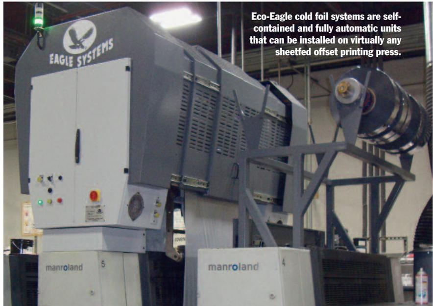
Eco-Eagle cold foil systems are self-contained and fully automatic units that can be installed on virtually any sheetfed offset printing press.
